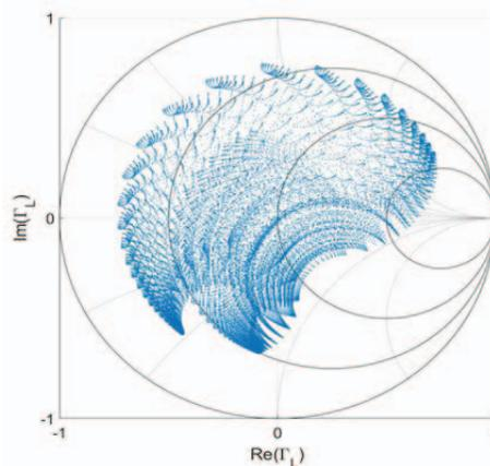
Fig. 2. Characterized load reflection coefficient states for the tunable varactor matching network
