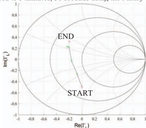
Fig. 6. Fast load-impedance optimization for output power from starting location  $\Gamma_L = 0.50/-90.0^\circ$ . A maximum  $G_T = 10.92$  dB was obtained at  $\Gamma_L = 0.38/122^\circ$  with 16 experimental queries.
