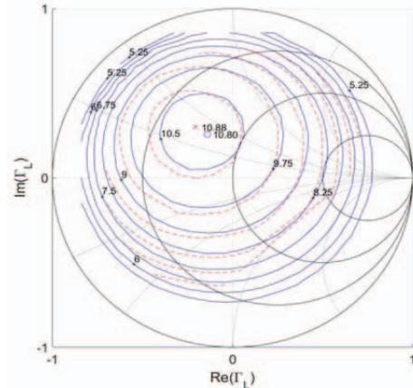
Fig. 5. 1.3 GHz single-tone MWT-173 FET load-pull transducer gain ( $G_T$ ) contours measured using the tunable-varactor matching network (dashed curves, optimum  $G_T = 10.88$  dB at  $\Gamma_L = 0.36/124^\circ$ ) and Maury load-pull tuner (solid curves, optimum  $G_T = 10.80$  dB at  $\Gamma_L = 0.29/118^\circ$ ) for -20 dBm input power.
