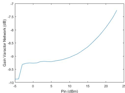
Fig. 3. Measured  $|S_{21}|$  versus input power for the varactor matching network at  $\Gamma_L = 0.7/90^\circ$ .
