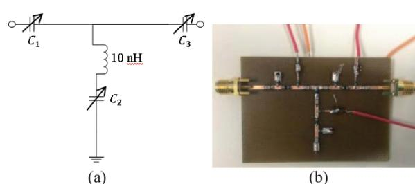
Fig. 1. (a) Design of 1.3 GHz tunable matching network, based on Fu [1], (b) implemented tunable-varactor matching network
