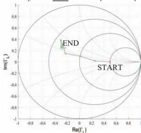
Fig. 7. Fast load-impedance optimization for output power from starting location  $\Gamma_L = 0.50/0^\circ$ . A maximum  $G_T = 10.87$  dB was obtained at  $\Gamma_L = 0.34/134^\circ$  with 33 experimental queries.
