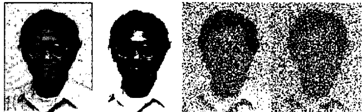
Figure 1. A simple example of stochastic resonance. The picture on the left is subjected to additive noise and is then thresholded. No noise (second from the left) and too much noise (on the right) render the image unrecognizable. At an intermediate resonant noise level, though, coarse structure is recognizable.
