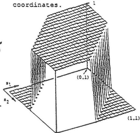
Figure 4. The generalization of the XOR networks formed by thresholding the function in Fig.3 at 3/4. Different hidden layer nonlinearities result in different generalizations.
