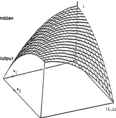
Figure 3. Response of the elementary XOR APNN using an exponential and trigonometric nonlinearity in the hidden layer. Note that, at the corners, the function is equal to the XOR of the coordinates.
