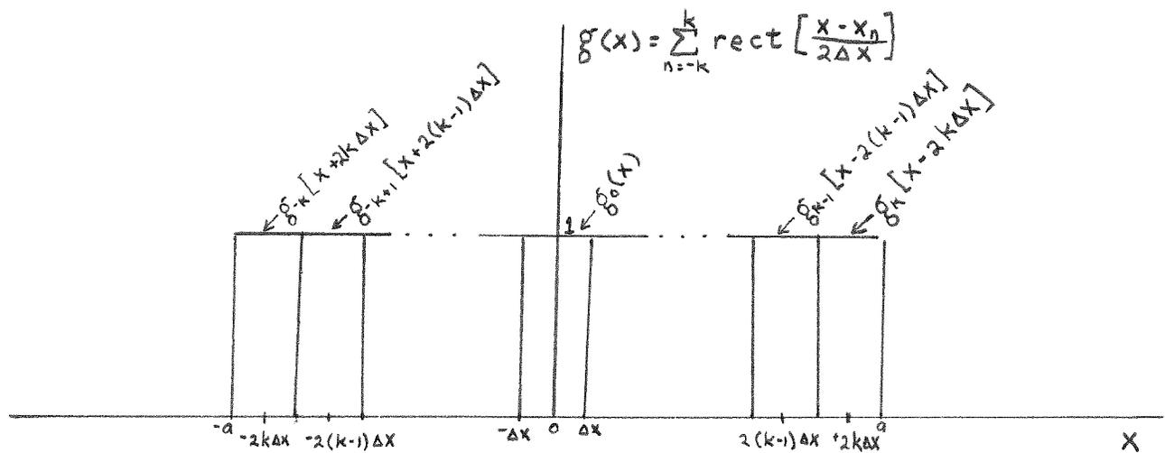
b) Dividing the input in (a) into isoplanatic patches. Each patch has width  $2 \Delta X$ .
