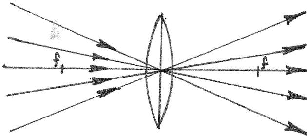
c) All rays passing through the lens at the lens axis remain unbent.
