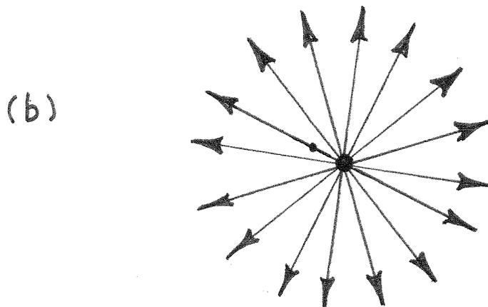
Fig. 3 : Spherical waves from a point source.
