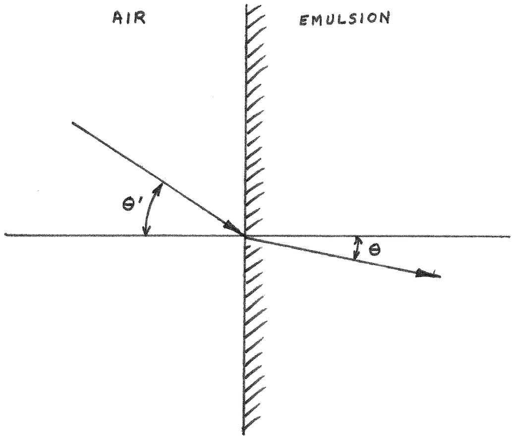
Fig. 19 : Illustration of Snell's law. The ray, entering a medium of homogeneous refractive index  $n$  from air with a refractive index of unity, is bent toward the normal in accordance with (2-98)
