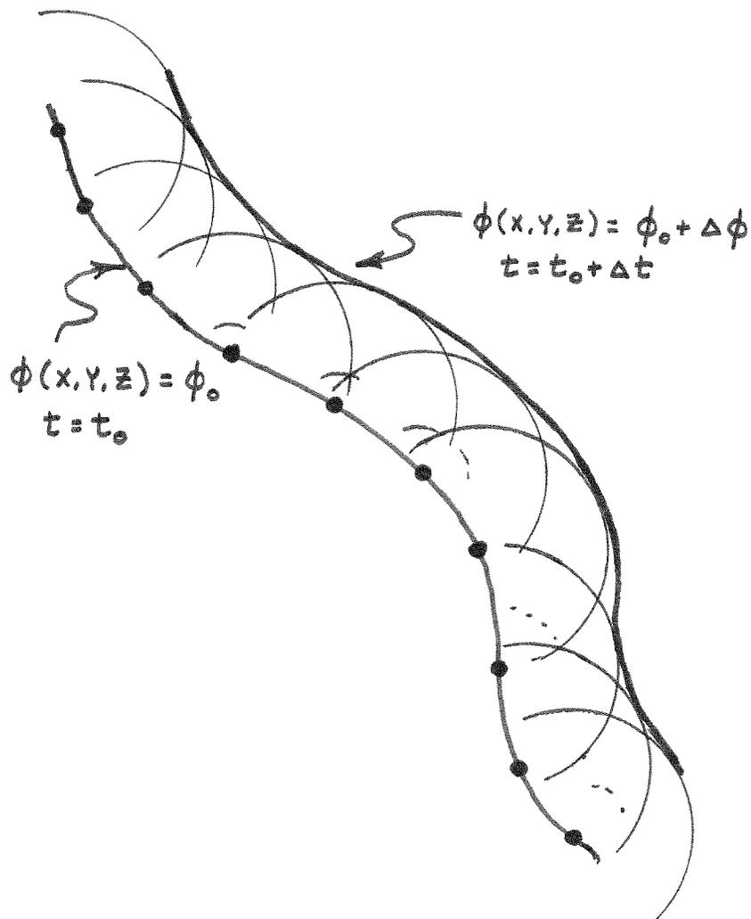
Fig. 5 : Illustration of the Huygens - Fresnel Principle. A wavefront at time  $t_0$ , ( $\phi(x, y, z) = \phi_0$ ) may be modeled as a continuum of secondary sources. The envelope of the resulting spherical wavelets after time  $\Delta t$  gives the position of the wavefront at time  $t_0 + \Delta t$ , ( $\phi(x, y, z) = \phi_0 + \Delta\phi$ ).
