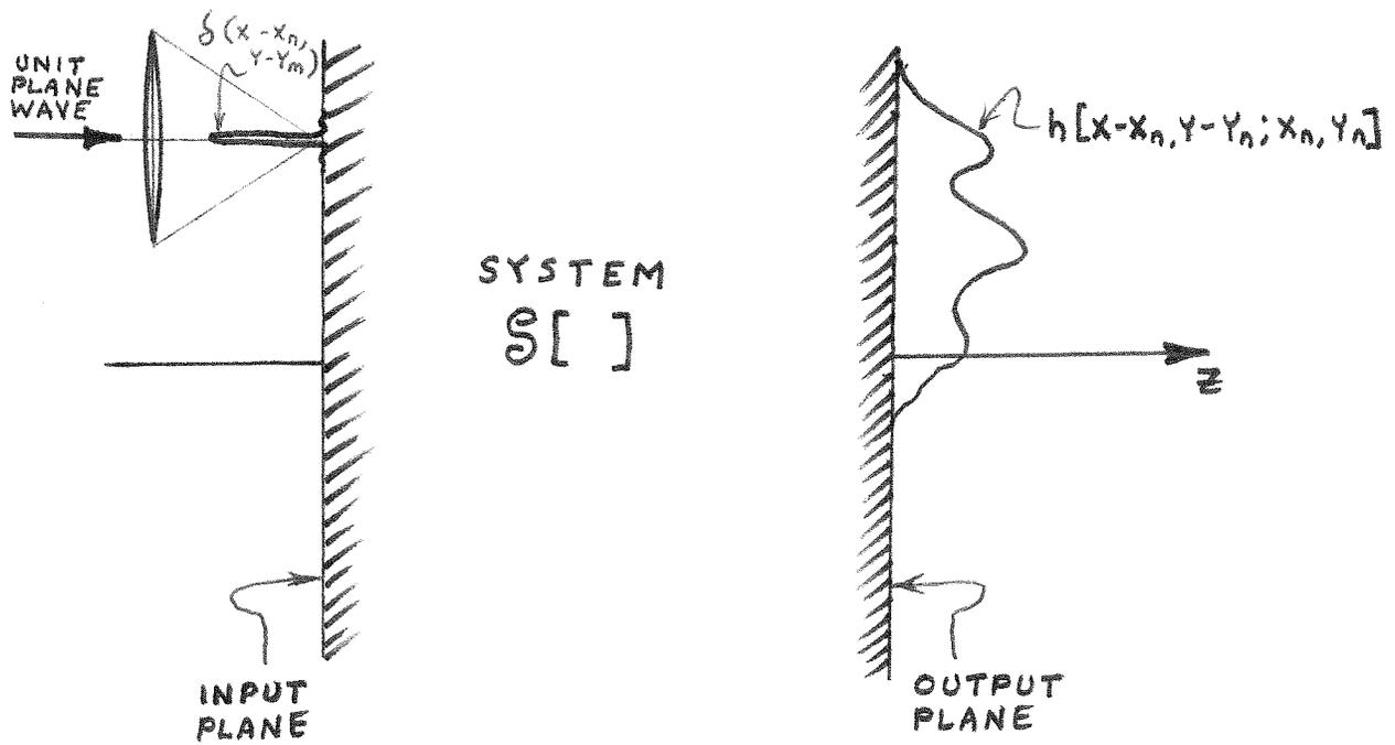
Fig. 30 : Generating a system's point spread function. A point source is focused at co-ordinates  $(x_n, y_m)$  of the system's input plane. The resulting distribution on the output plane is  $h_{nm}(x-x_n, y-y_m)$ .
