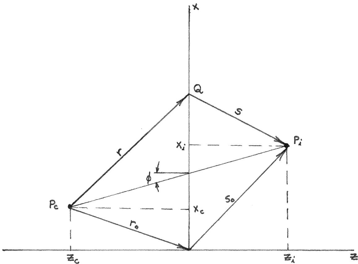
Fig. 17 : The geometry describing the two dimensional Fresnel - Kirchoff integral in equation ( 2-48).
