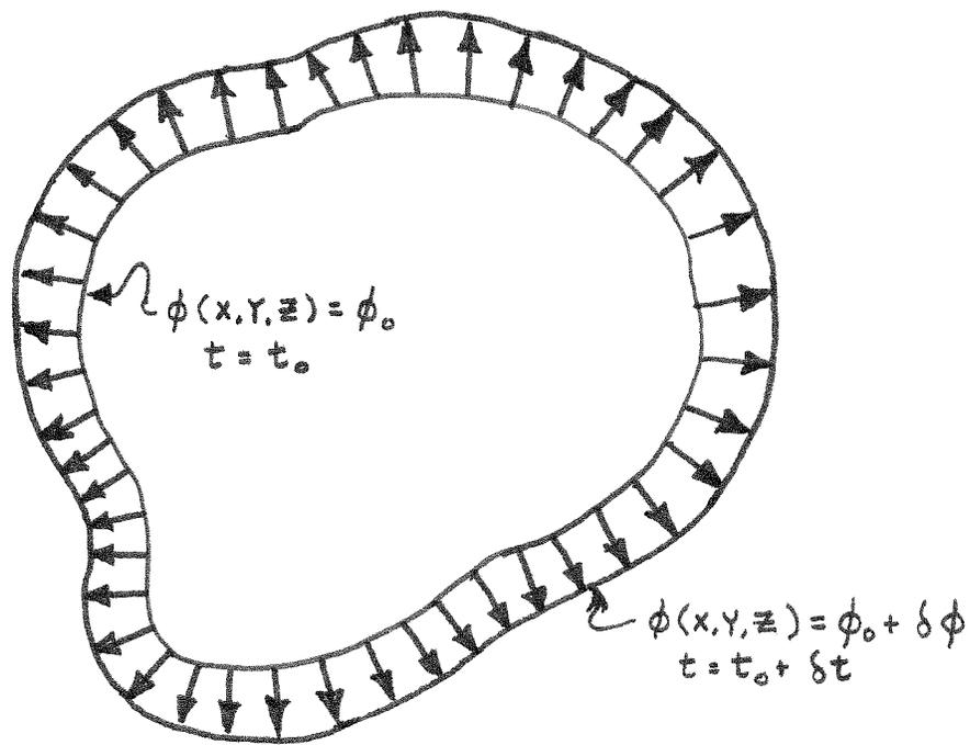
Fig. 2 : Equiphase surfaces or wave fronts,  $\phi(x, y, z)$  at times  $t_0$  and  $t_0 + \delta t$ . The point by point mapping of the inner to outer surface is established by the rays.
