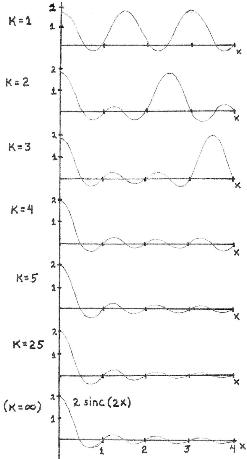
Fig. 27 : Piecewise isoplanatic approximated output of a Fourier Transformer with an input  $\text{rect}[x/2]$  as given by (3-108). The input pulse was divided into  $2k+1$  isoplanatic patches. The true output is  $2 \text{sinc}(2x/\lambda f)$ . (The above curves are for  $\lambda f = 1$ )
