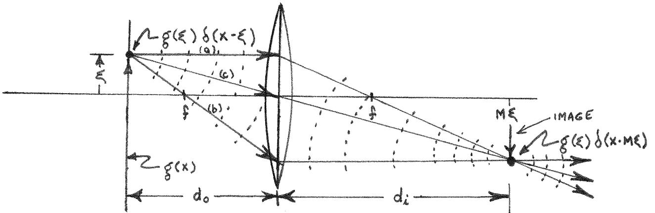
a) Magnifier when  $d_o > f$ . The image is inverted ( $M < 0$ ) and real.
