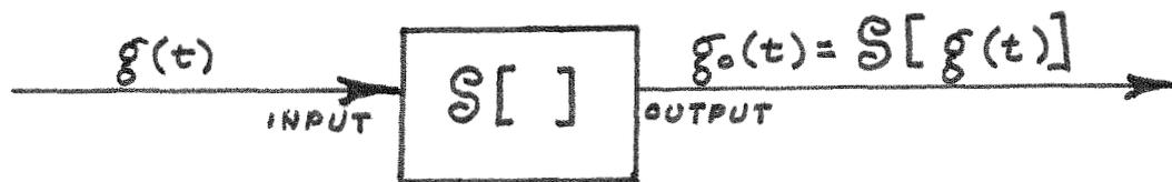
Fig. 22 : The general system model consisting of an input, a system described by the mathematical operator  $S[ ]$ , and an output.
