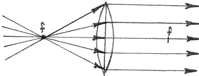
b) All rays passing through the front focal point emerge parallel to lens axis.
