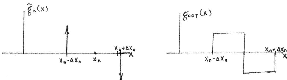
Fig. 42 : Comparison of outputs of left; piecewise isoplanatic approximation and right; theoretical output of a macroscopically thick system recording.
