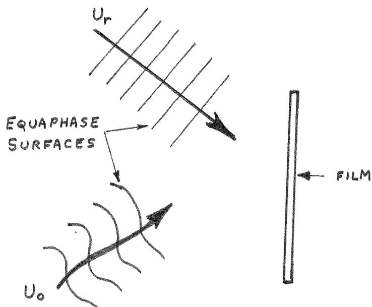
Fig. 10 : Holographic recording results from two beating waves. The reference wave ( $U_r$ ) chosen here as planar, is recorded simultaneously with an object wave, ( $U_o$ ) depicted here by wave equiphase surfaces to illustrate its more arbitrary nature.
