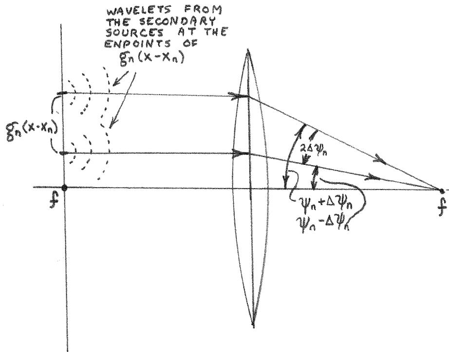
Fig. 33 : The maximum angular interval from an isoplanatic region is centered at  $\psi_n$  and has a width of  $\Delta\psi_n$ .
