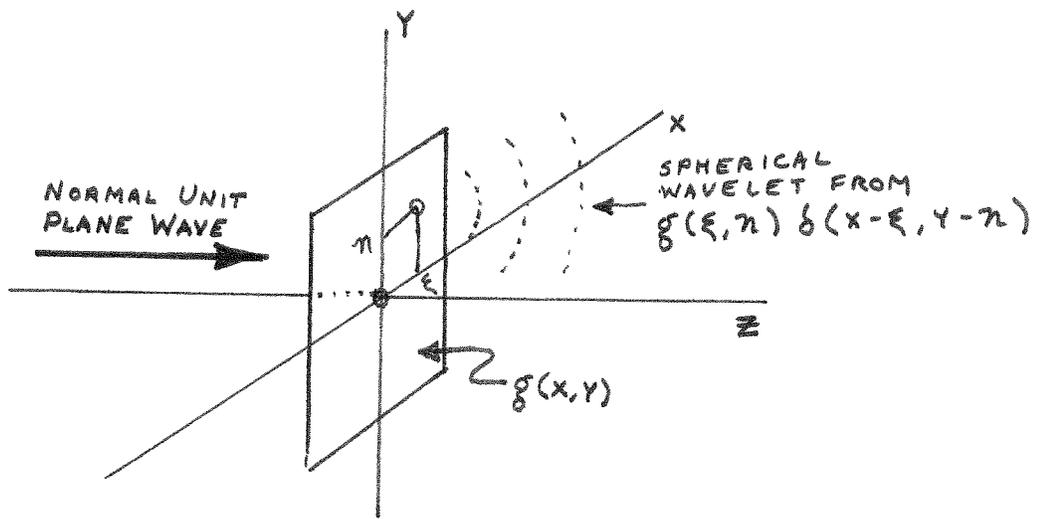
Fig. 6 : Application of the Huygens - Fresnel Principle to a transmittance, each point on  $g(x, y)$  acts as a secondary source.
