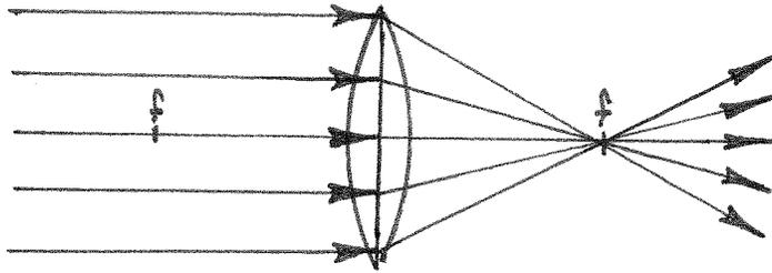
a) All rays parallel to the lens axis pass through the back focal point.
