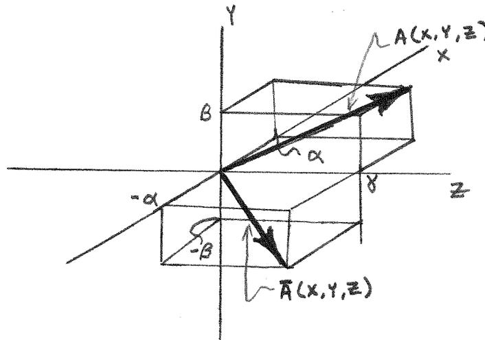
b) The alternate conjugate ray for the case where one is concerned solely with the distribution on the X - Y plane. Note the equivalent X and Y components of the conjugate unit amplitude ray here and in Fig. 7a.
