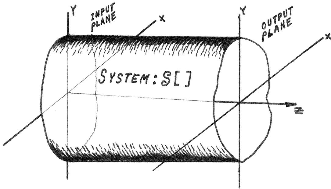
Fig. 23 : General portrayal of an optical system consisting of an input plane, a system, and an output plane.
