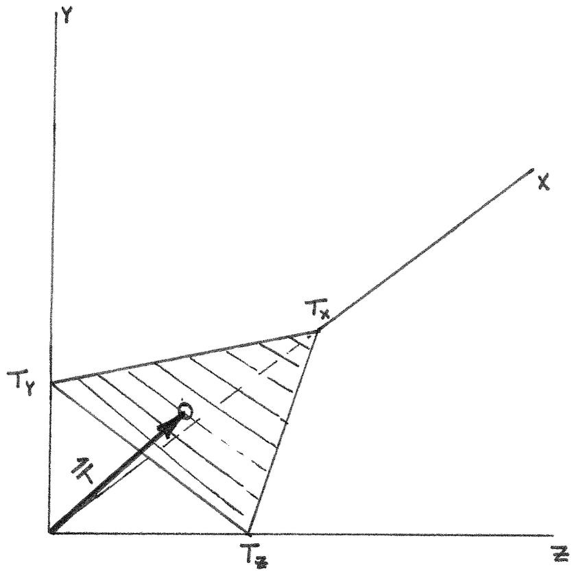
Fig. 13 : A plane of constant intensity formed by two beating plane waves. The perpendicular distance between two adjacent planes is given by the period vector  $\vec{T}$ .
