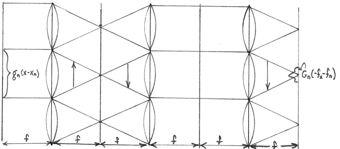
b) Transforming with three fly's eye lenses to invert the resulting Fourier Transform of the input  $g_n(x-x_n)$ .
