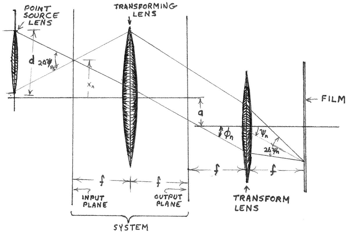
Fig. 37 : System recording of the Fourier Transformer after the more general Fig. 36.
