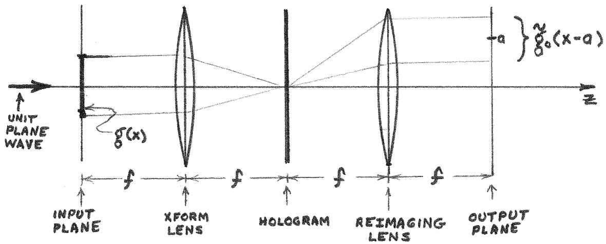
Fig. 35 : Desired reconstruction geometry for implementation of the piecewise isoplanatic approximation employing the extinction angle.
