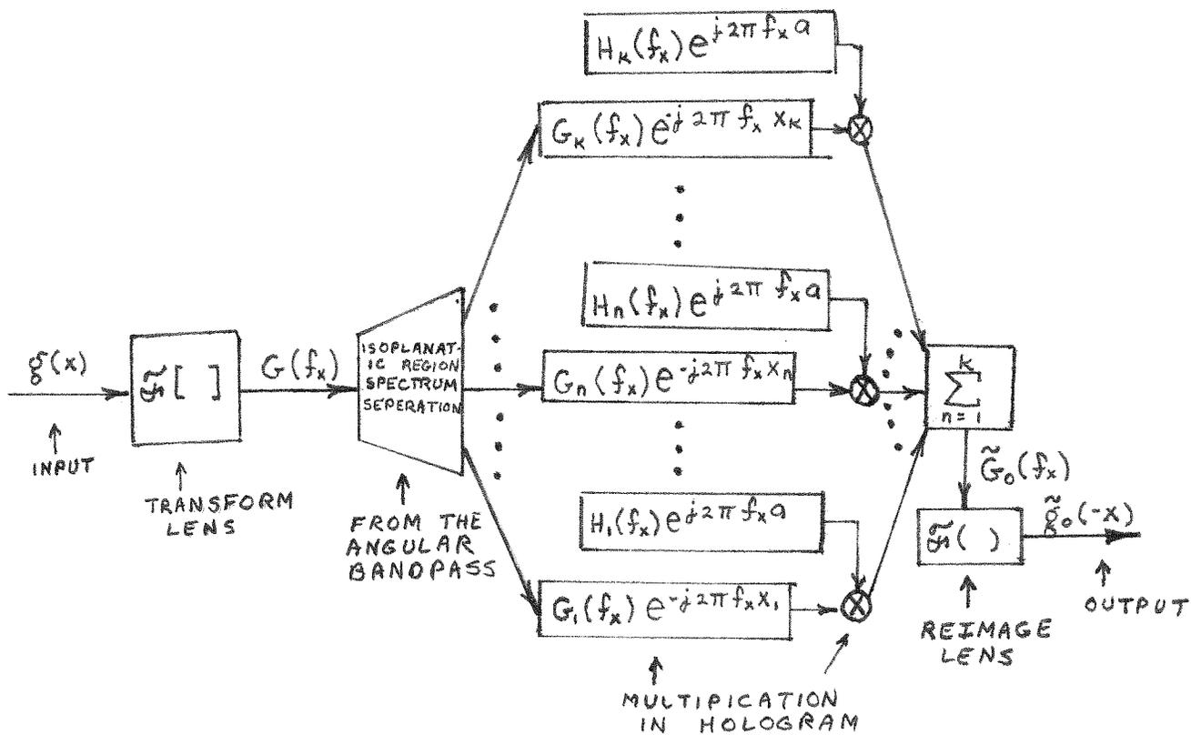
Fig. 43 : Block diagram of the extinction angle recording method fullfilling the piecewise isoplanatic approximation.
