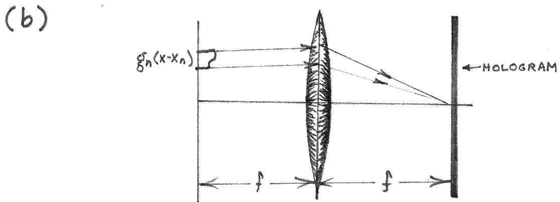
Fig. 41 : (a) Recording and (b) reconstruction with a macroscopically thick hologram. Note the equivalent angular interval of the transformed "rect" reference beam in (a) and the transformed isoplanatic region in (b). This assures alignment of the angular bandpass.
