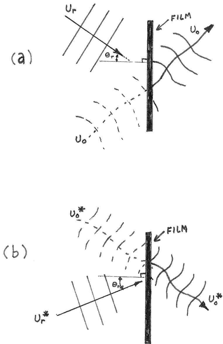
Fig. 12 : Illustration of wavefront reconstruction.
