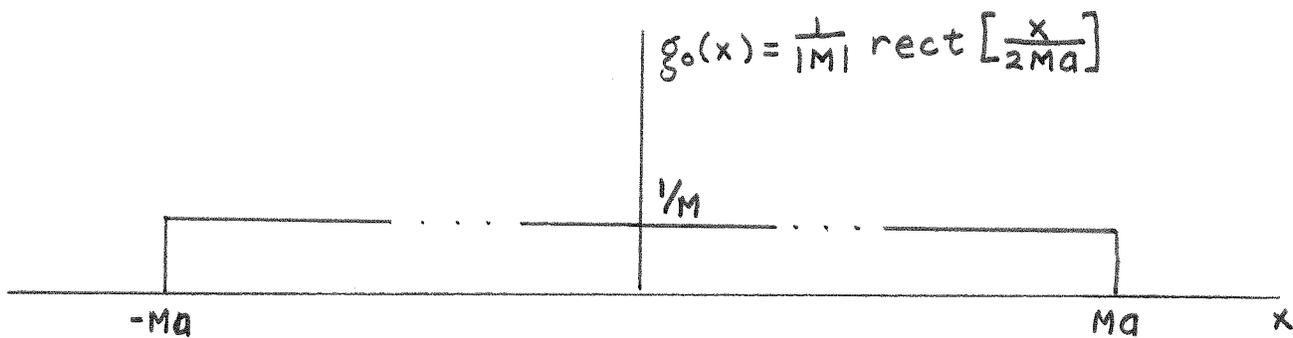
c) The true output for the simple magnifier for the input given in (a).
