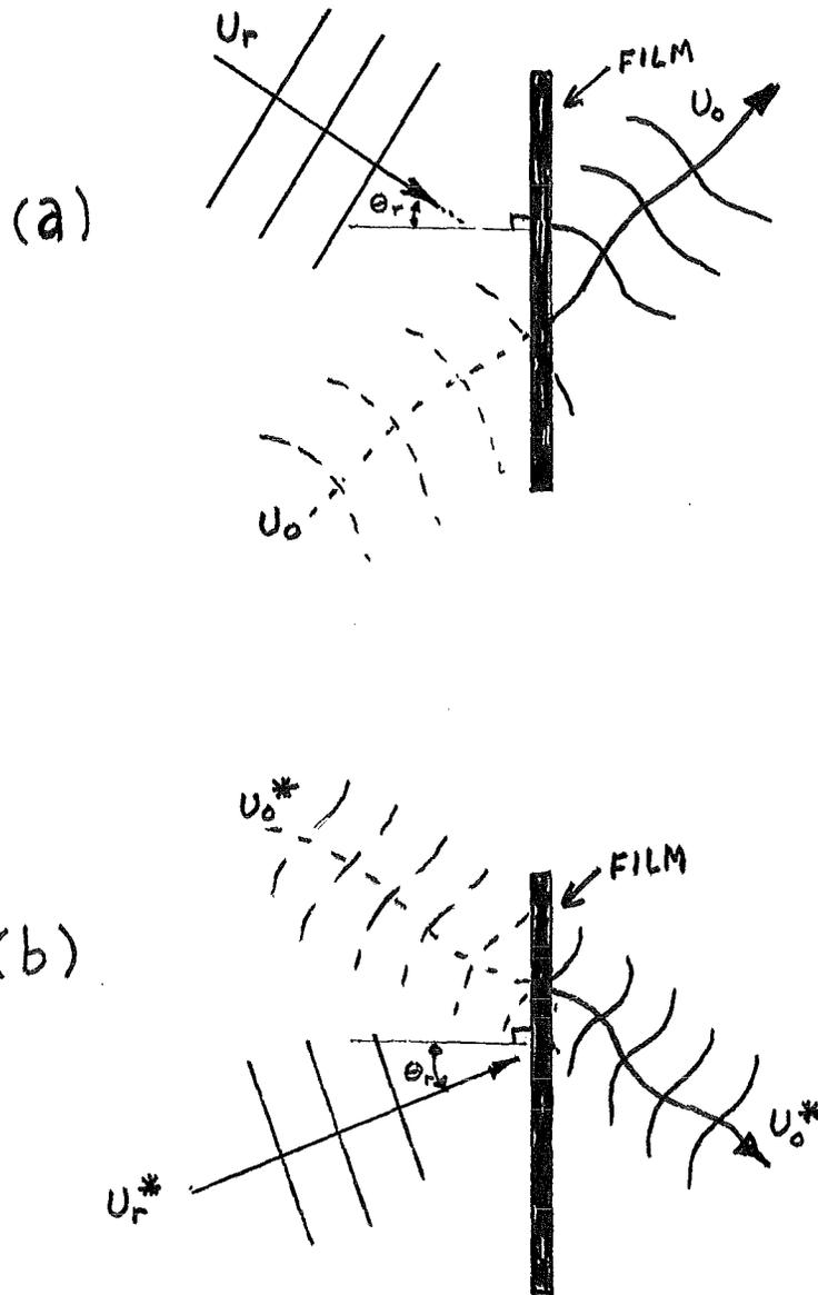
Fig. 12 : Illustration of wavefront reconstruction.
