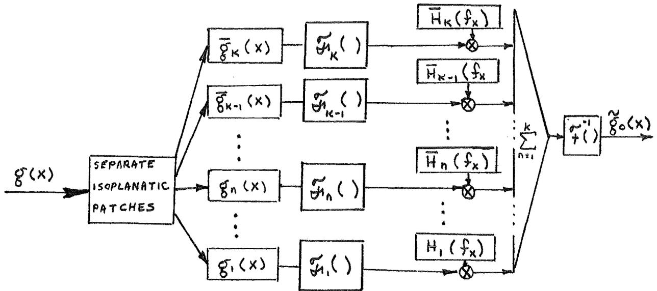
Fig. 45 : Alternate system synthesis scheme for implementing the piecewise isoplanatic approximation. All isoplanatic regions are Fourier Transformed in some manner and are multiplied by a corresponding transfer function. All processed patches are summed and transformed to give the system's approximated output.
