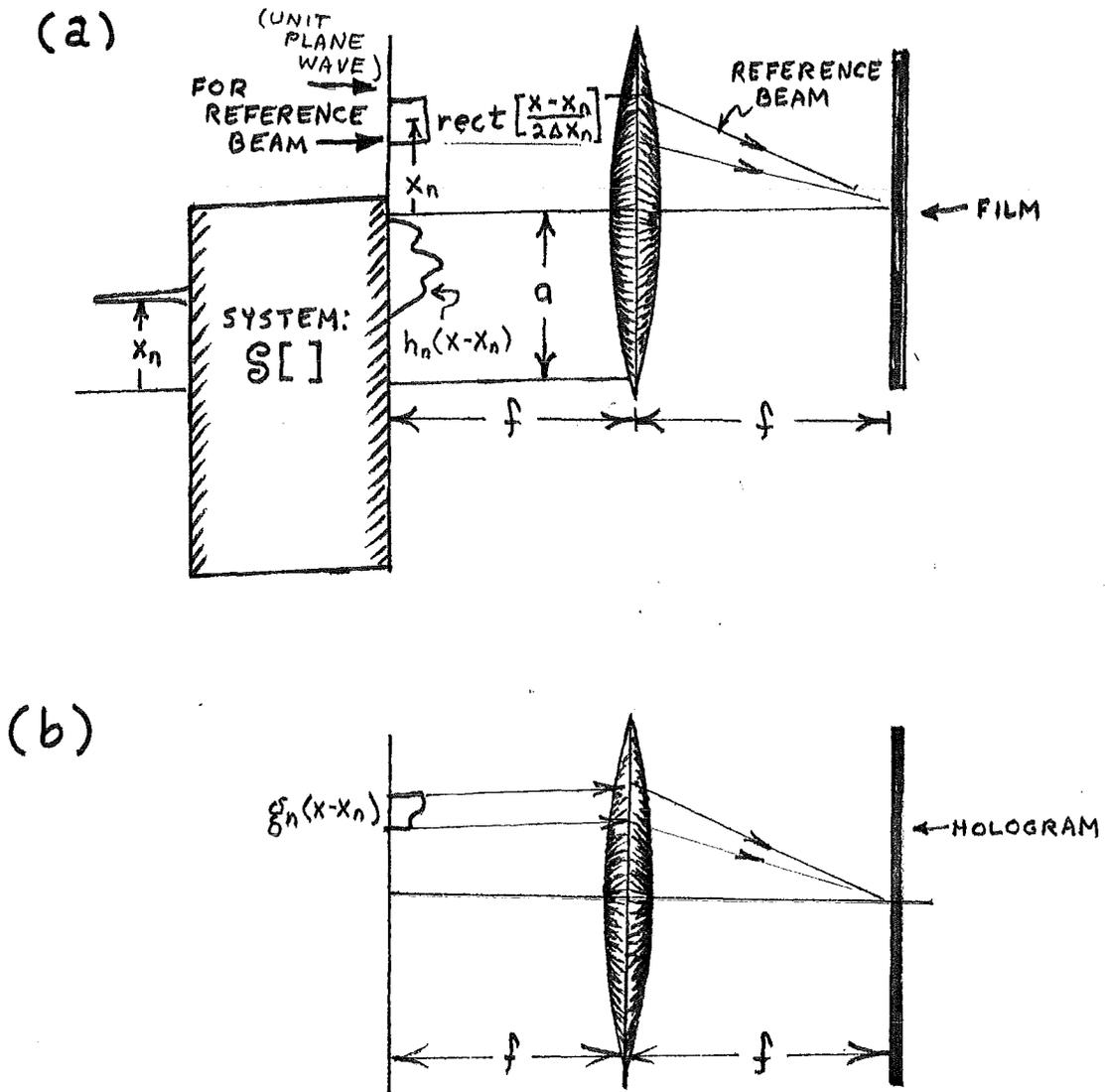
Fig. 41 : (a) Recording and (b) reconstruction with a macroscopically thick hologram. Note the equivalent angular interval of the transformed "rect" reference beam in (a) and the transformed isoplanatic region in (b). This assures alignment of the angular bandpass.
