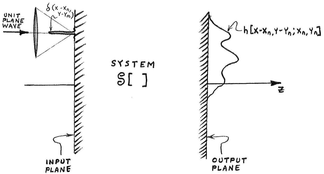
Fig. 30 : Generating a system's point spread function. A point source is focused at co-ordinates  $(x_n, y_m)$  of the system's input plane. The resulting distribution on the output plane is  $h_{nm}(x-x_n, y-y_m)$ .
