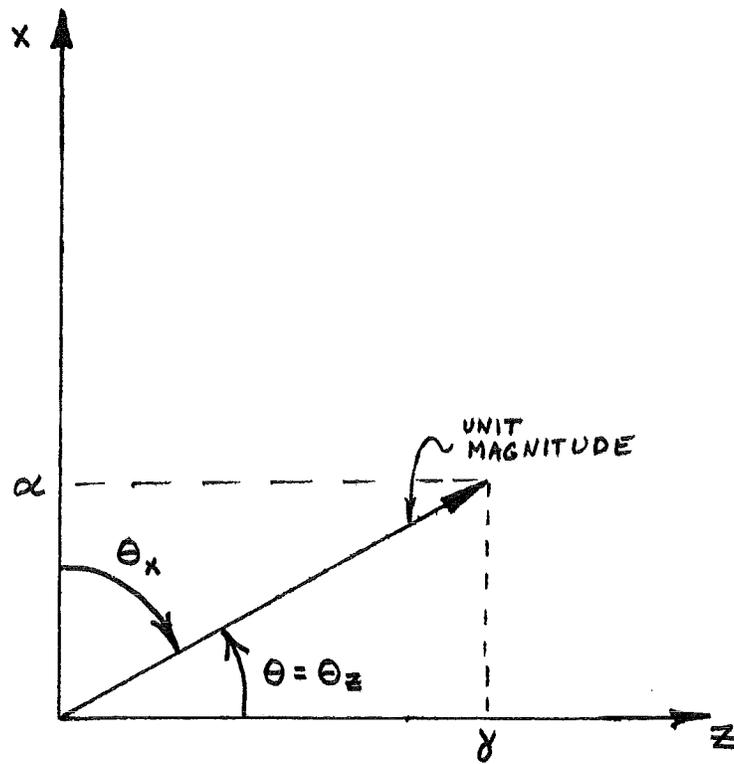
Fig. 15 : Relationship of the direction cosines ( $\alpha$  and  $\gamma$ ) in two dimensions.
