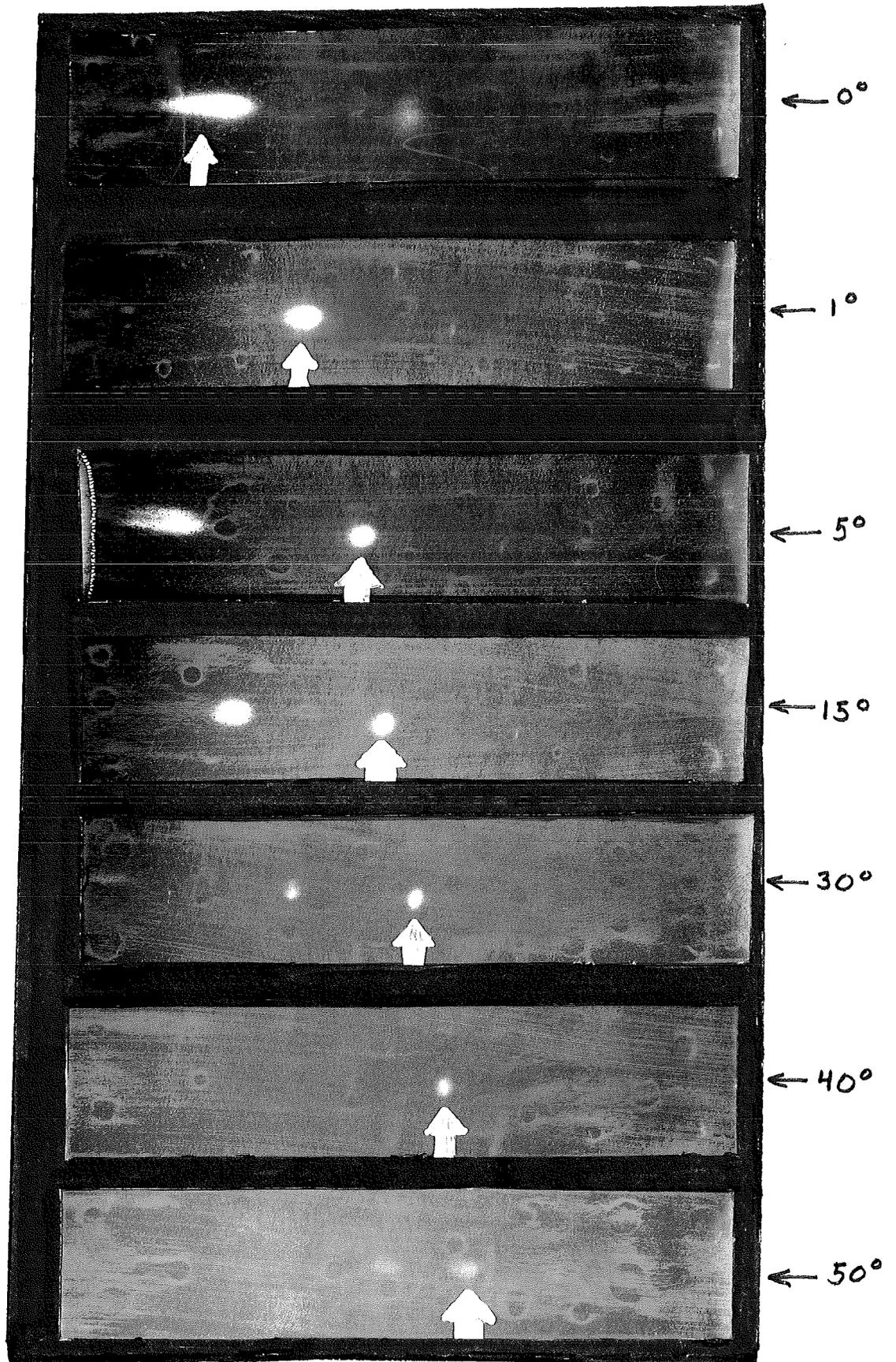
Fig. 48 : Distortion from diffracted waveforms from a binary grating as a function of reconstruction angle.
