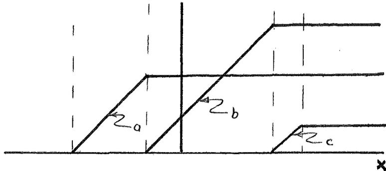
ii) Corresponding processed patches. Each ramp has a slope of unity.
