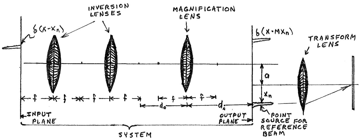
Fig. 38 : Extinction angle recording geometry for the non-inverting magnifier after the more general Fig, 36.
