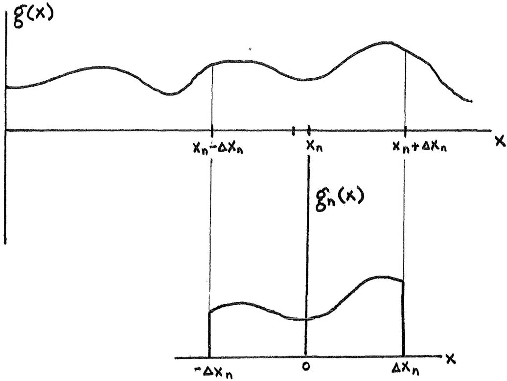
Fig. 24 : Extraction of the  $n$ th isoplanatic region from  $g(x)$ .
