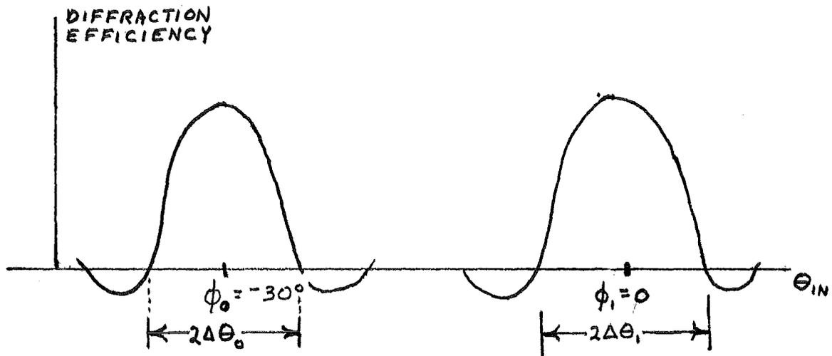
c) Resulting diffraction efficiency.
