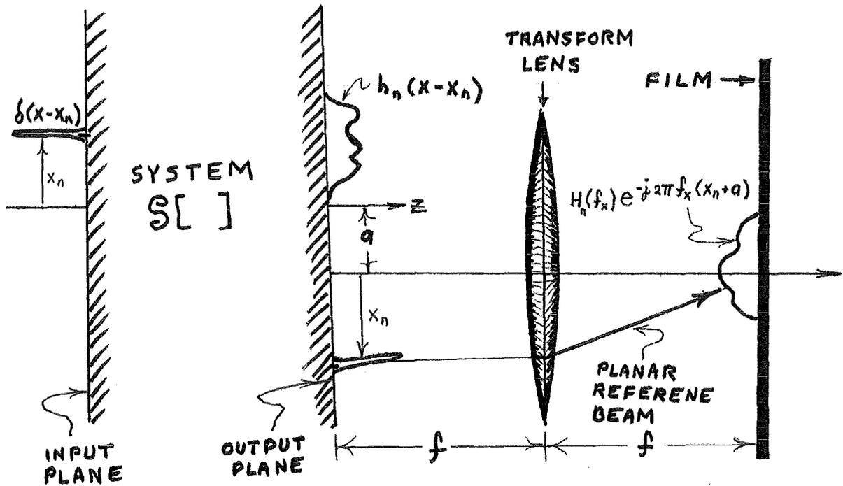
Fig. 36 : Holographic recording of the transfer function expression given by (4-42).
