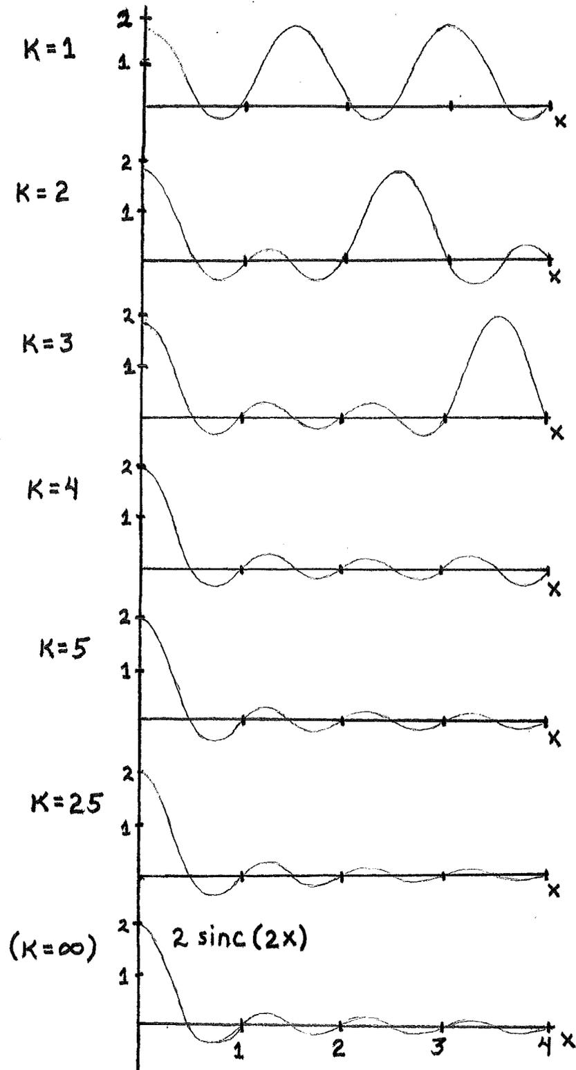
Fig. 27 : Piecewise isoplanatic approximated output of a Fourier Transformer with an input  $\operatorname{rect}[x/2]$  as given by (3-108). The input pulse was divided into  $2k+1$  isoplanatic patches. The true output is  $2 \operatorname{sinc}(2x/\lambda f)$ . ( The above curves are for  $\lambda f = 1$  )
