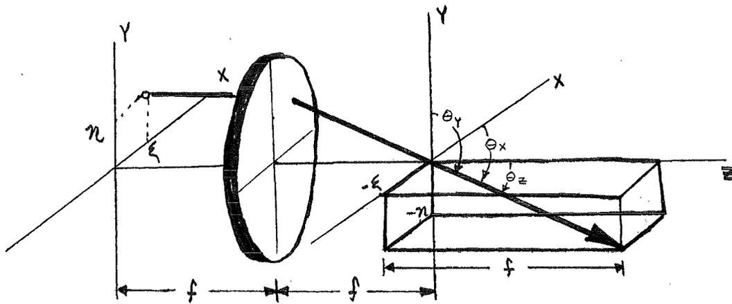
Fig. 9 : Collimation of a point source located in the front focal plane of a double convex thin lens three dimensions. The resulting propagation direction of the plane wave is defined by  $\theta_x$ ,  $\theta_y$  and  $\theta_z$ .
