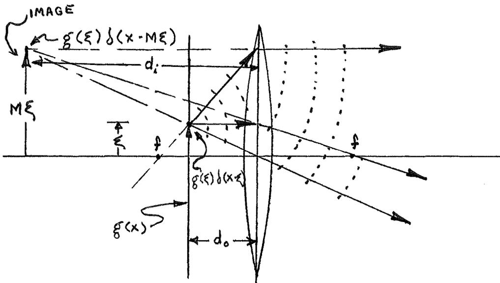
b) Magnification when  $f < d_o$ . The image is erect ( $M > 0$ ) and virtual.
