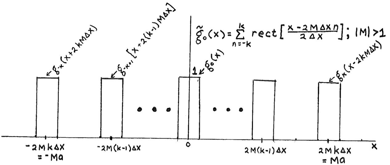
d) Piecewise isoplanatic approximated output for the simple magnifier for  $|M| > 1$ . Each pulse has width  $2\Delta x$ .
