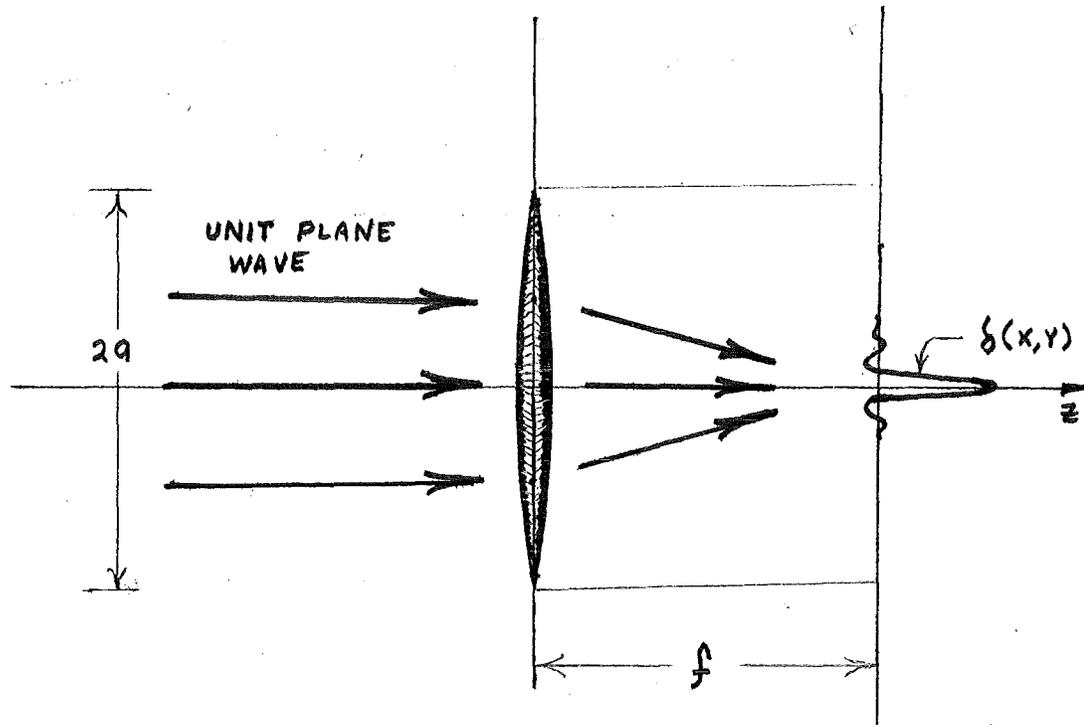
Fig. 29 : Generating the dirac delta by focusing a plane wave to a point source on the back focal plane of a thin lens.
