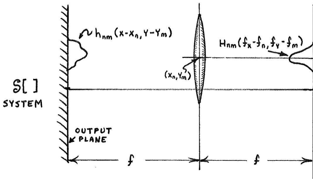
Fig. 31 : Two methods to generate transfer function expressions. The point spread function, as generated in Fig. 30, is Fourier Transformed by a thin lens placed at co-ordinates
