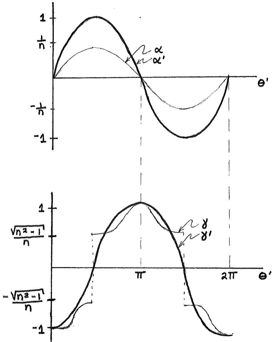
Fig. 21 : Refractive index limitations placed on the direction cosines within a recording medium of refractive index  $n$ . Primed variables denote the corresponding direction cosines external to the medium.
