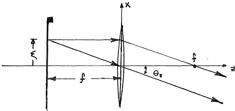
Fig. 8 : A point source on the front focal plane is collimated by the double convex thin lens to a plane wave.
