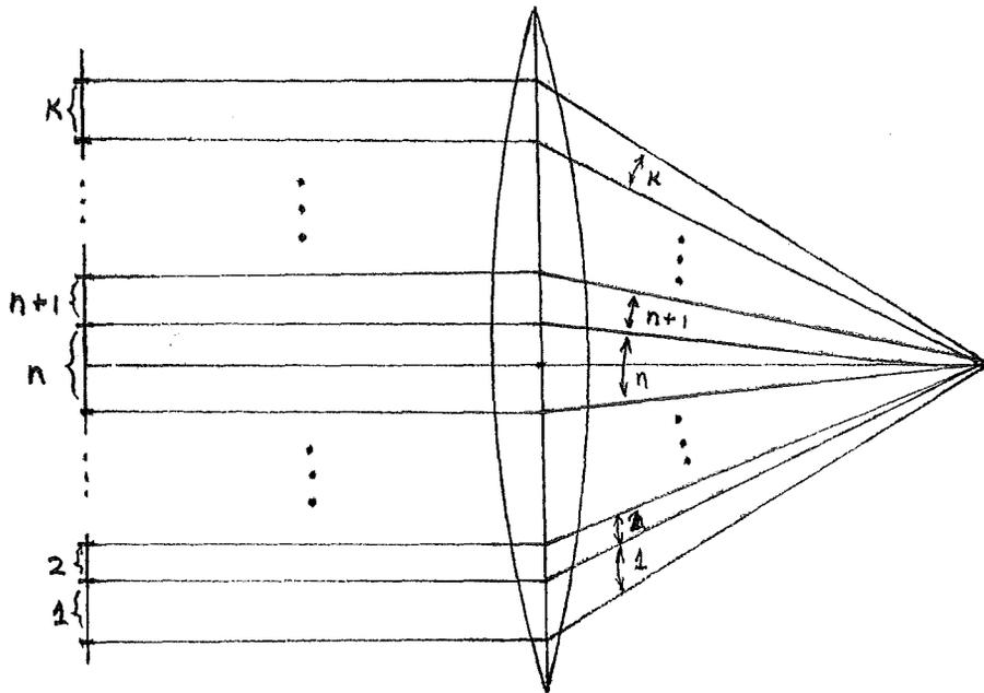
Fig. 44 : Mapping of block orthogonal isoplanatic regions to block orthogonal intervals.
