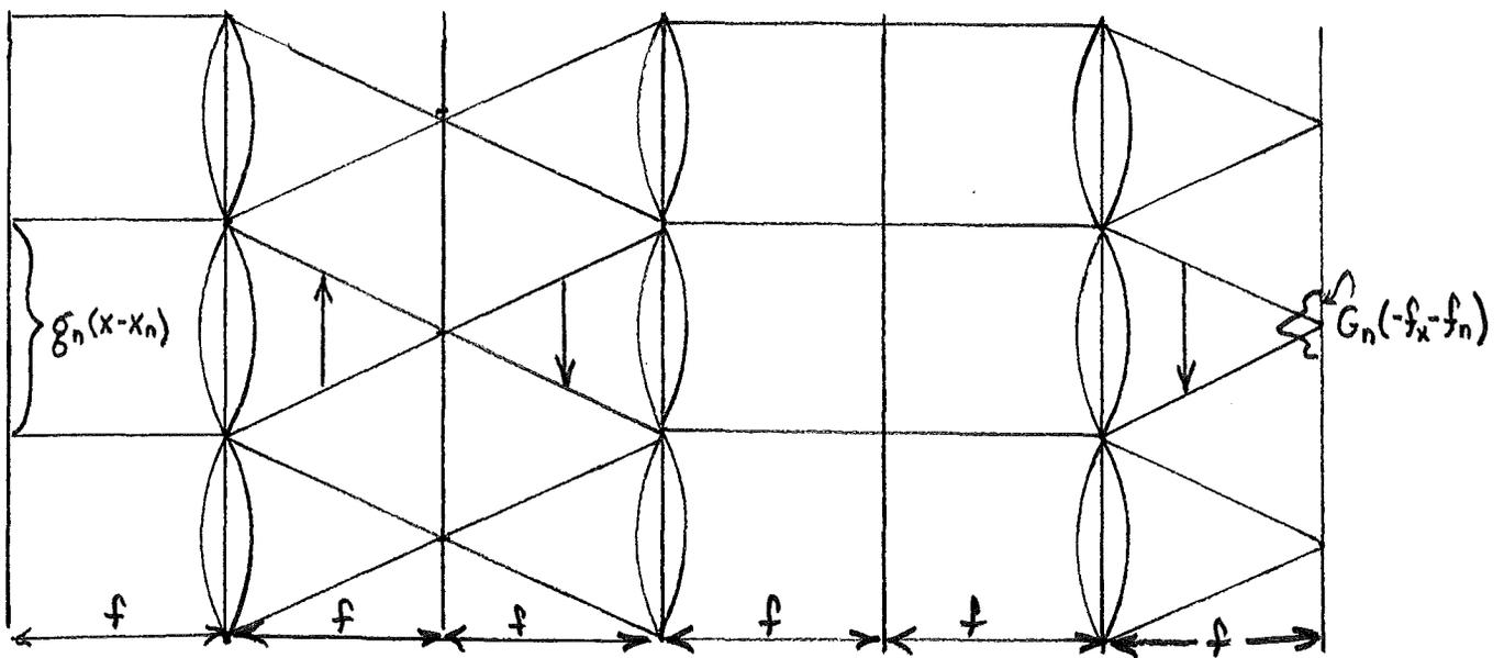
b) Transforming with three fly's eye lenses to invert the resulting Fourier Transform of the input  $g_n(x-x_n)$ .
