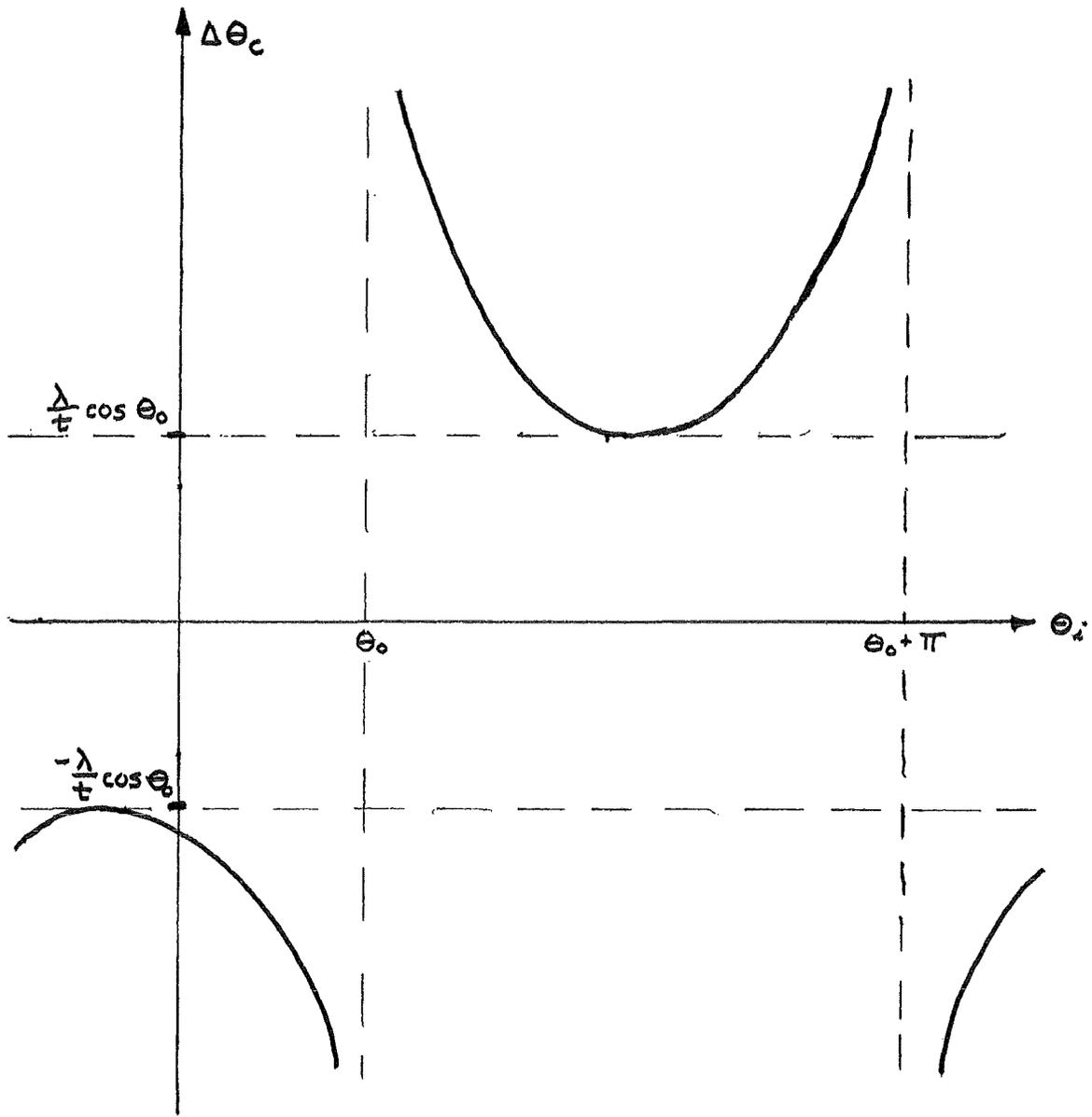
Fig. 18 : A first order approximation of the extinction angle as a function of the angle of incidence of the reconstruction beam.
