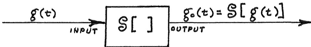
Fig. 22 : The general system model consisting of an input, a system described by the mathematical operator  $S[ ]$ , and an output.
