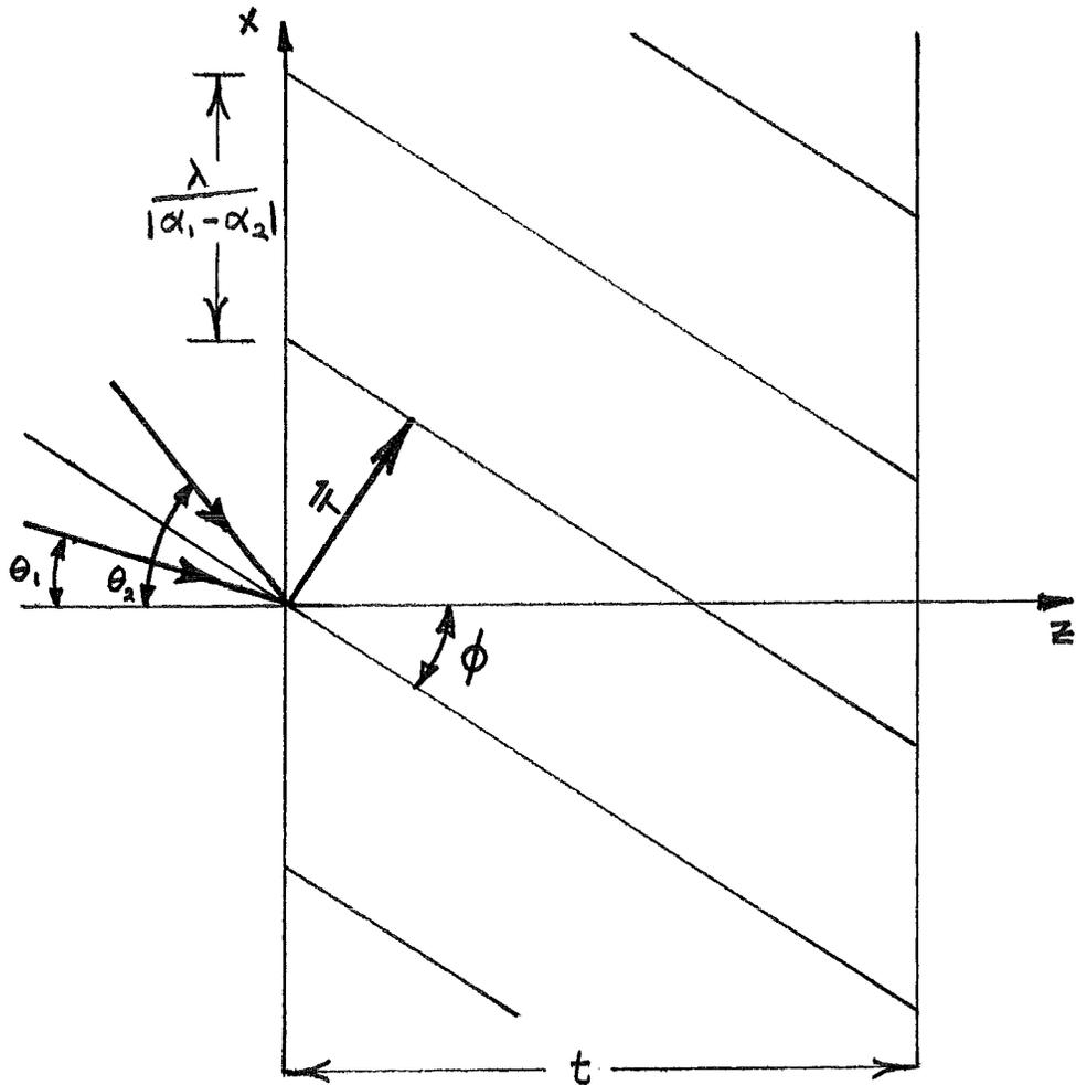
Fig. 14 : Geometry of the maximum intensity loci in a volume hologram formed by two plane waves propagating at angles  $\theta_1$  and  $\theta_2$  with respect to the hologram's normal.
