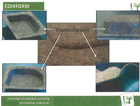
**Figure 8. Excellent formability in compression molding of non-woven fabric composites with 50 wt% coir.**
