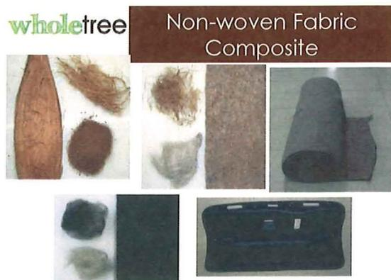
**Figure 7. Creation of a trunk lid by substituting coir for polyester in the non-woven fabric composite of polyester-polypropylene that is compression molded into various trunk trim parts.**
