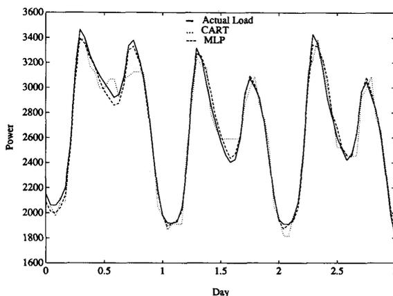
Fig. 2. A comparison of the performance of an MLP and CART (with linear combinations) in predicting three days of hourly power loads in megawatts.
