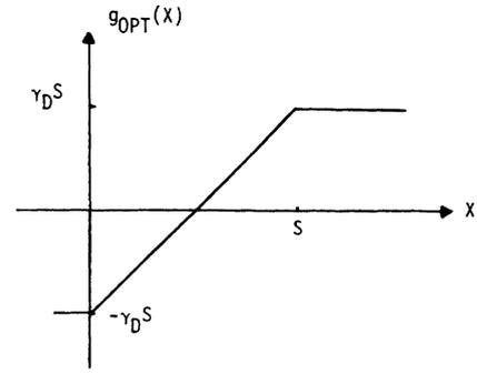
Fig. 2. MNL for the optimal detector.
