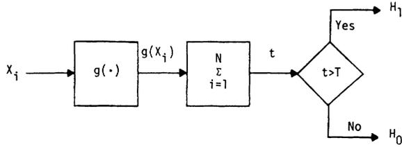
Fig. 1. Standard form of a detector.
